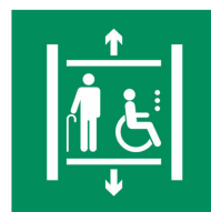
Figure 21. Examples of special escape signs for accessibility according to ISO 7010 and DIN EN 81-76
