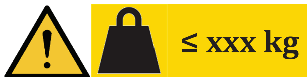
Figure 2 — Maximum permissible load on a platform
