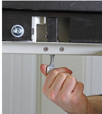
Car door lock engaged when the car is outside the landing door area
