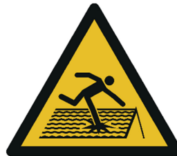
Figure 18 — Not walkable roof
